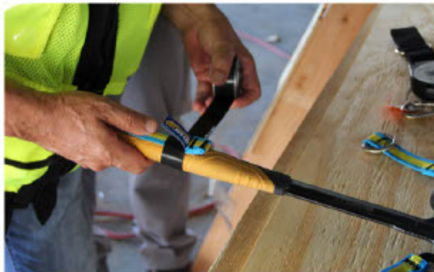
ToolMate® Link Strap Attachment with D-ring (RTM-LS2.25) used with Attachment Tape (RTM-LTR)
