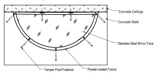
NOTE: When installing with tamper proof fasteners, it is important to eliminate damage to the mirror face and powder-coated frame.
