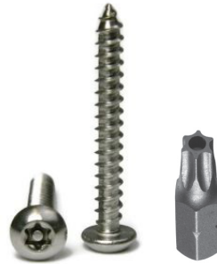
Button Head Torx Security Masonry Screw Size: 1/4" x 1 3/4" (6.35mm x 44.45mm) Driver Size: #27 Torx Security 1/4" (6.35mm) Hex Bit Drill Dia: 3/16" (4.76mm)
