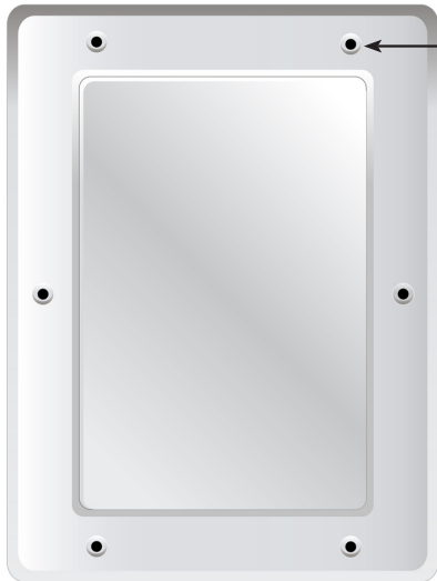
Button Head Torx Security Masonry Screw Size: 1/4" x 1 3/4" (6.35mm x 44.45mm) Driver Size: #27 Torx Security 1/4" (6.35mm) Hex Bit Drill Dia: 3/16" (4.76mm)
