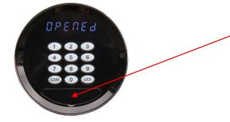
Initially the keypad may not have batteries fitted. To insert the batteries, pull the door open, remove the grey cover from inside the drawer and load 4pcs 1.5V AA Alkaline batteries. Replace the battery cover.
